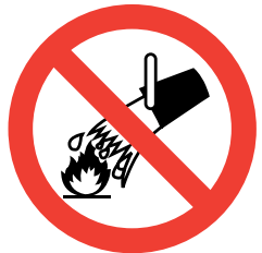
Do not extinguish with water
